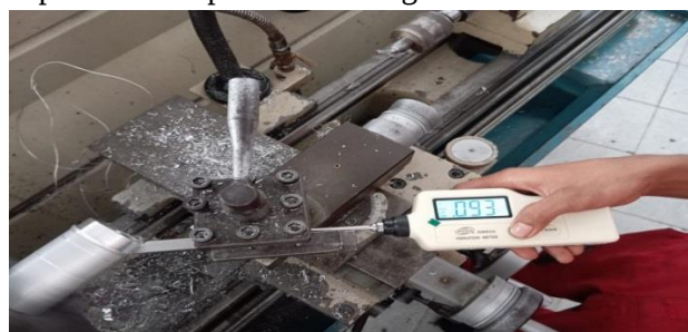
Fig. 1. Experimental setup for turning and vibration measurement
