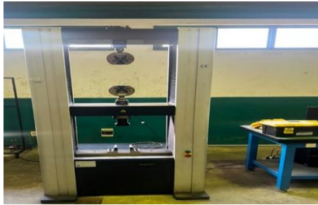
Fig 6. Experimental Setup of the Three-Point Bending Test for Honeycomb Rib Specimens with a 130° Polygon Angle
