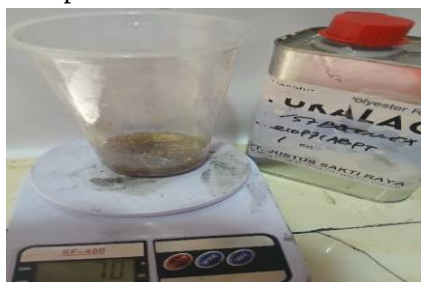
Fig 2 pouring 70% polyester resin
