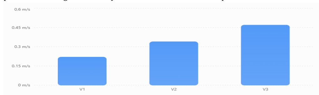
Fig 4. Comparison of average air velocity at each variation of air inlet position.
