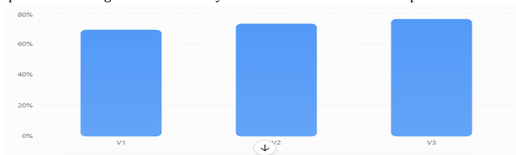
Fig 3. Comparison of average relative humidity at each variation of water inlet position.
