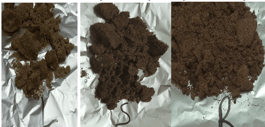
Fig 2. Acetylated biosorbent of from the leaf, stem and root of cissus populnea plant for sorption studies.
