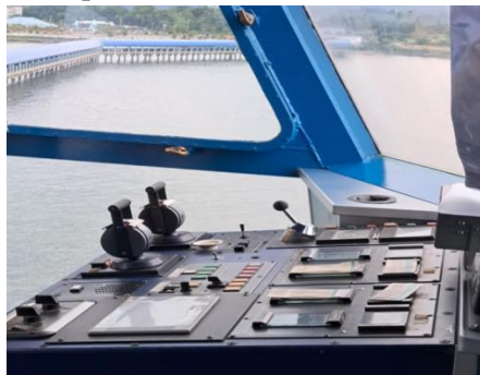
Fig. 3 Manual Steering (Left Side) Docking Platform
