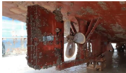
Figure 9 Documentation of the Condition of the Ship's Rudder Leaf
