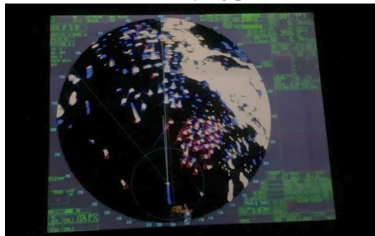
Fig. 1 X-Band Radar on LPG/C Gas Arar ship
