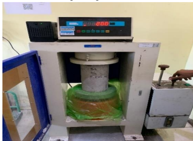
Fig 4. Compression Testing Machine (CTM).
