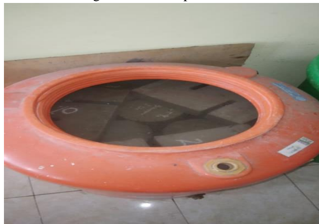
Fig 3. Concrete test body maintenance.
