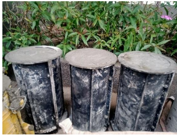
Fig 2. Manufacture of cylindrical test pieces.
