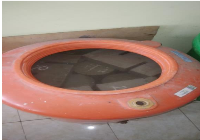
Fig 3. Concrete test body maintenance.
