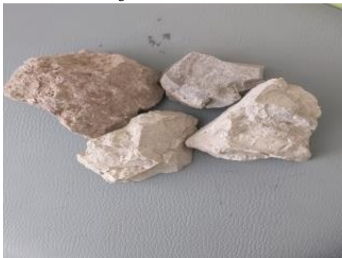
Fig 1. Uncrushed raw bentonite clay
